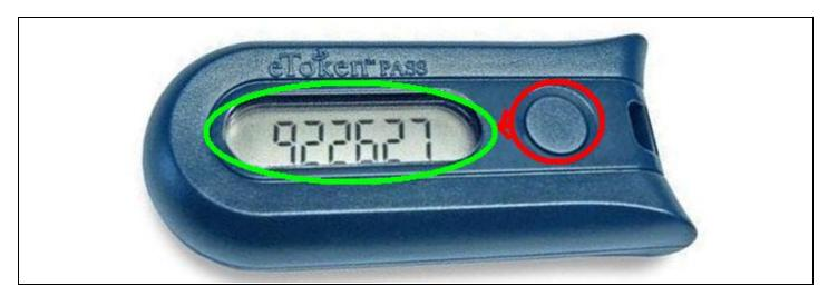
The Hardware OTP Token will then show the currently generated OTP code on its LCD display. Copy this OTP code into the relevant field in IB.
